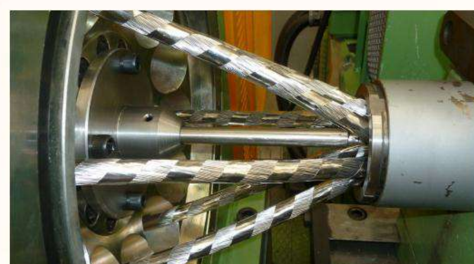
Manufacture of CICC: cabling higher stage (courtesy of L. Muzzi, ENEA)
